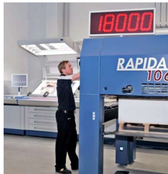
Closed-loop quality production on a KBA Rapida 106 with QualiTronic Color Control and INSTRUMENT FLIGHT®
