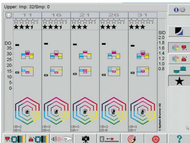
The HEXAGON* diagrams used for the control methods INSTRUMENT FLIGHT* inline-online and PRODUCTION-CHECKER online/offline. A maximum of 5 stars rate the degree of conformity to the selected print standard.
