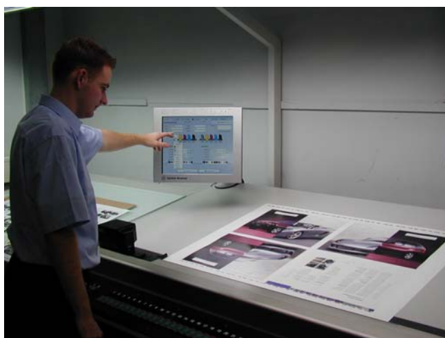
INSTRUMENT FLIGHT* online with Touchscreen operation from the MAN Roland control console: Color consistency even with the most difficult subjects.
